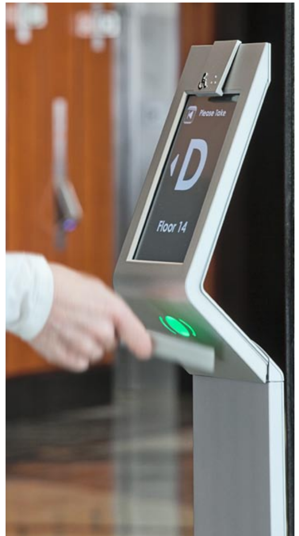
Photo left: Don Carter, principal in Raleigh Development Company. Photo below: PORT devices incorporate RFID card readers that direct tenants to elevators that will take them to their destination floors with the fewest number of stops.
